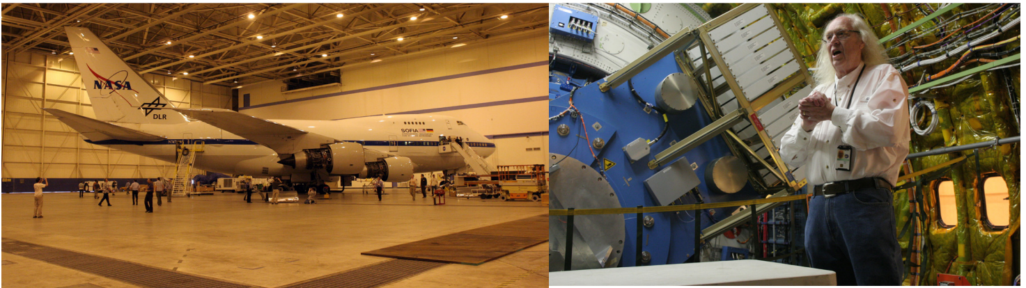
Left: Things got off to a flying start with a tour of the Stratospheric Observatory for Infrared Astronomy (SOFIA) at its home base in Palmdale—though the plane remained in its hangar. Right: Inside the aircraft, SOFIA chief scientist Eric E. Becklin (UCLA) described the observatory's 2.5-meter telescope, situated behind the cabin's aft bulkhead and instrument interface, seen at left.
